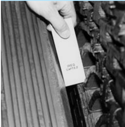
1986 – Air gap sensor developed at IREQ, shown next to a generator air gap.
