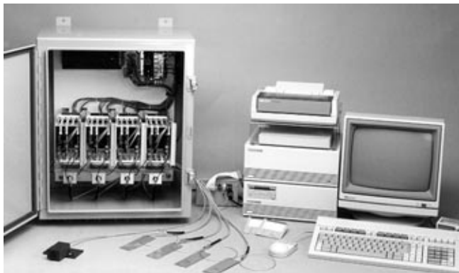
1986 – First generation AGMS commercialized: 4-ch acquisition unit, air gap sensors designed at IREQ, and PC running on HP-DOS.
