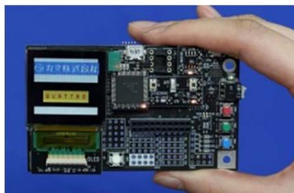
Original sensor solution evaluation board for IoT
