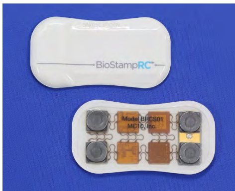
MC10社製 Flexible Wearable Bio Sensor BioStamp®
