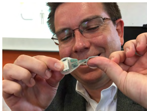
MC10社製 Flexible Wearable Bio Sensor BioStamp®
