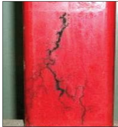
Electrical tracking of high voltage bus due to contamination
