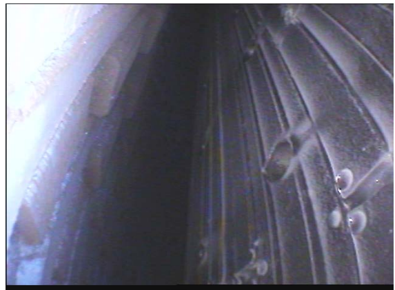
Figure 17: Drive End - Air Gap with Dirt and Oil
