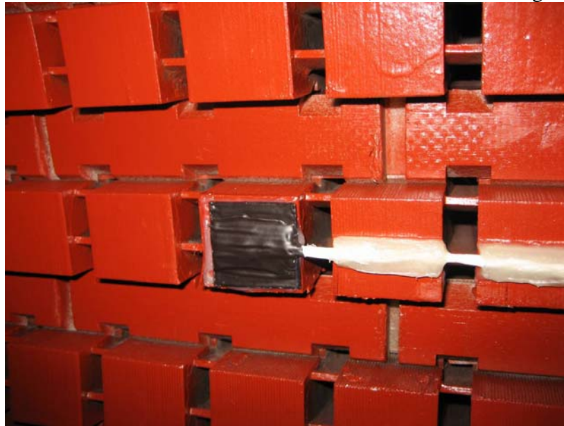
Figure 1. Total Flux Probe™ mounted on a tooth
