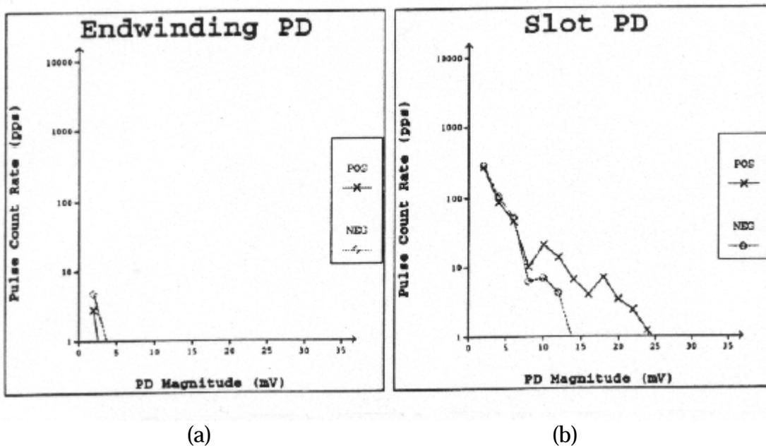
Figure 8 PD activity in the slot and endwinding with the Turkey Point Unit 1 generator operating at 460 MW.
