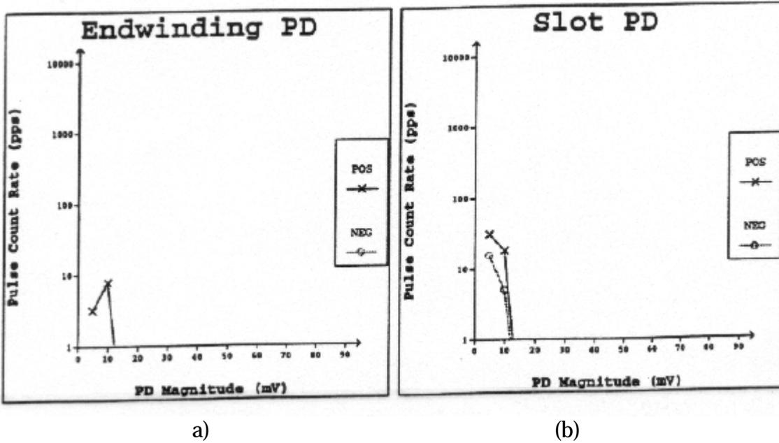
Figure 7 PD pulse height analysis plots for an SSC installed in a new 122 MVA generator.
