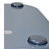
Dual antenna RTK-GPS for accurate localization
