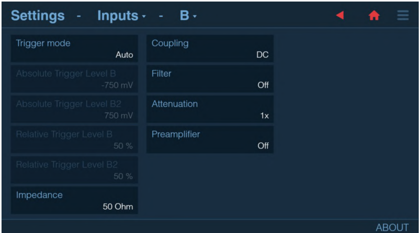
Figure 34. Example configuration for Time Interval A to A to B to B measurement
