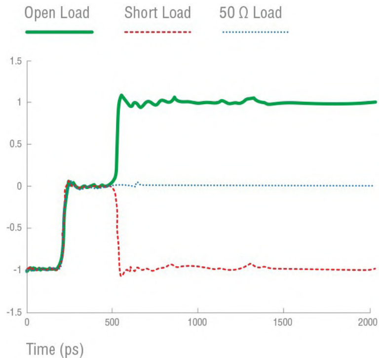
Figure 32. Measuring Time Interval between 2 levels of reflected signal in TDR measurement allows to calculate the distance to cable break
