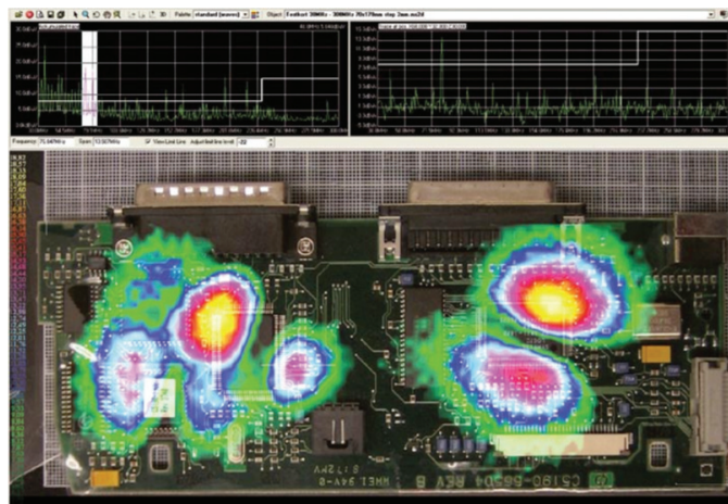
MultiScan measurement. The top left graph shows the accumulated trace (a max hold spectrum of all measuring points). The top right graph shows the wide band spectrum from a user selectable spot on the field plot.
