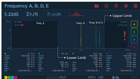
The Frequency distribution view reveals the spread (stability) of the oscillators
