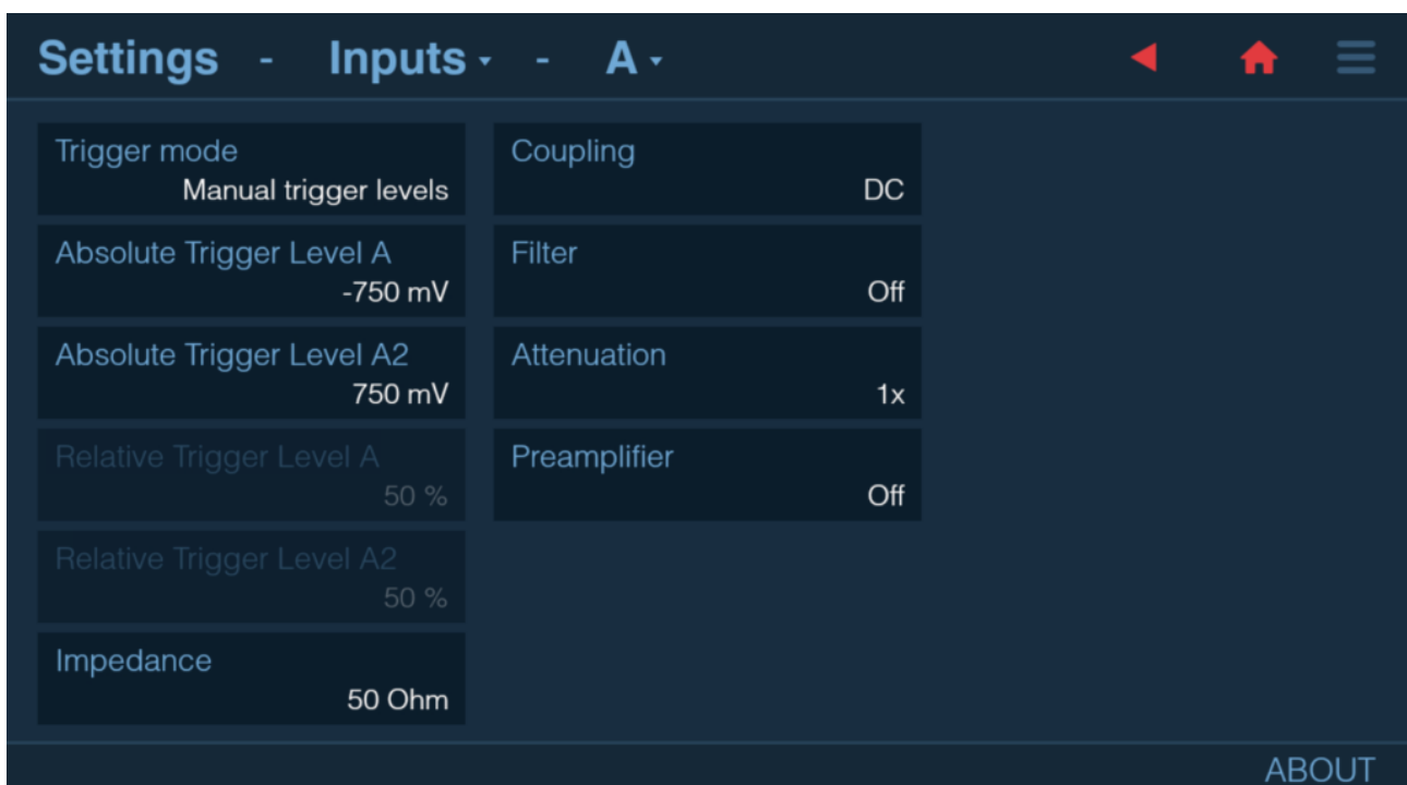
Fig. 5.9: Instrument's configuration for TDR measurement on Figure 28
