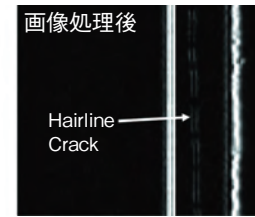
Post Imaging Processing Defect Image
