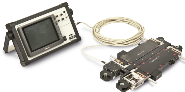
Robotic Inspection Vehicle (RIV) with camera—offline inspection and testing of the stator core with rotor in place
