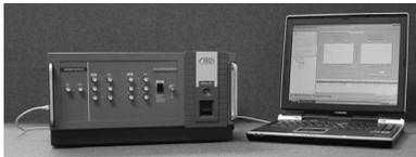
Portable instruments perform partial discharge tests on motors and generators on-line and off-line
