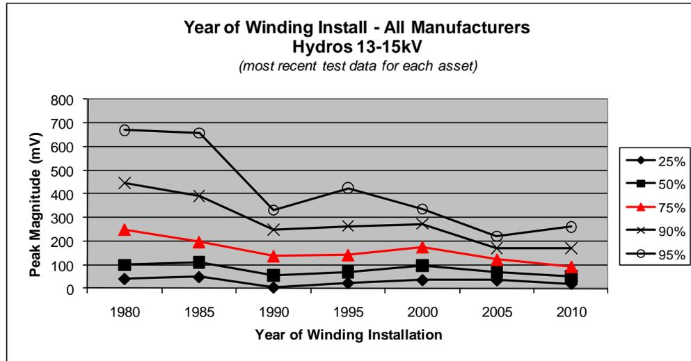
Chart 8. Hydros 13-15kV by Year of Install (test results of 2009)
