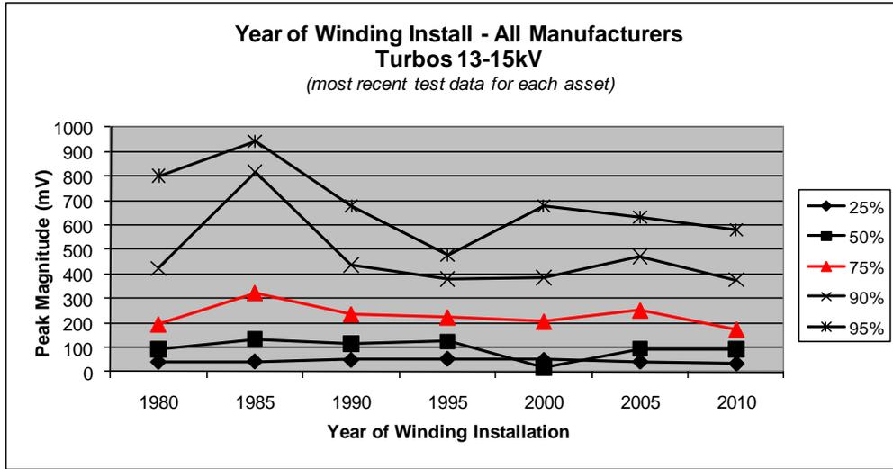
Chart 4. Turbos 13-15kV by Year of Install (test results of 2009)
