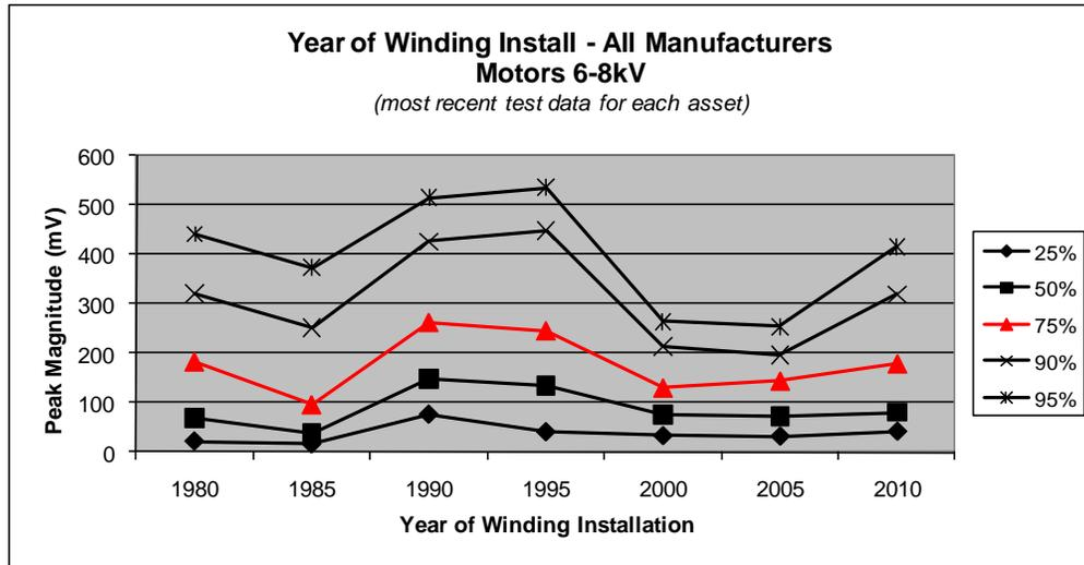
**Chart 2. Motors 6-8kV by Year of Install (test results of 2009)**
