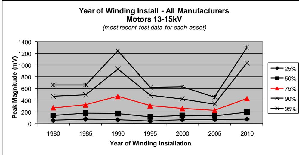
**Chart 6. Motors 13-15kV by Year of Install (test results of 2009)**
