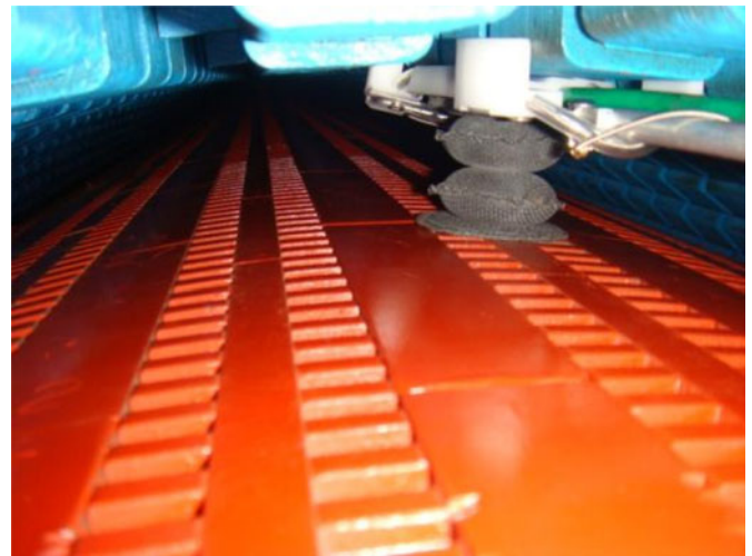
Fig. 10. TF probe installation with rotor in situ .
