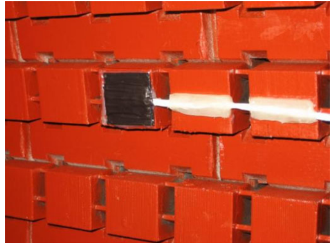
Fig. 9. Photo of installed TFProbe.
