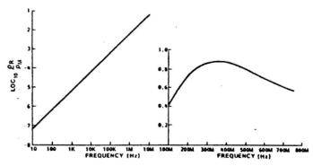
Fig. 4: The ratio of S/K for a rectangular bandpass (pR) to S/N for a matched filter  $p^{\wedge}$  as a function of the high frequency limit of the rectangular bandpass filter. A l.S ns FWHH Gaussian pulse input is assumed. Note the change from logarithmic to linear frequency scale at 100 MHz.
