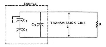
Fig. 5: Model for calculating the rise time of a partial discharge pulse for a solid dielectric sample in a transmission line. The HV pouer supply is not shown.
