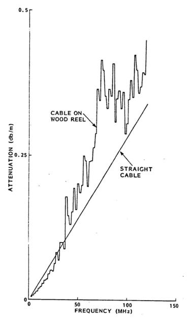
Fig. 8: Loss vs frequency for a typical 28 kV XLPE distribution cable manufactured without a copper tape ground shield. The loss for the reeled cable shows the effects of layer to layer coupling at high frequencies.
