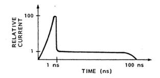
Fig. 2: Theoretical shape of a PD in a email void. The duration and magnitude depends on the void size, gas, electric field, etc. [9].
