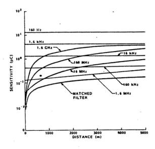
Fig. 9: Partial discharge detection sensitivity vs distance to the partial discharge source for the 28 kV distribution cable (Fig. B). These sensitivities are calculated for a 20 dB S/N.
