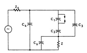
Fig. 6: Model for calculating the rise time Of a partial discharge pulse in a lumped element detection system.
