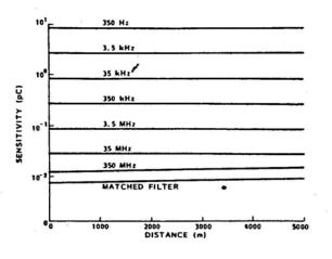
Fig. 7: Partial discharge detection sensitivity  $v\partial$  distance to the PD source as calculated for 500 kV GITL. These sensitivities are for a 20 dB S/N, assuming perfect amplifiere at 290 K. Real amplifiers will reduce the sensitivity by 2 to 10 dB. Note that a S/Nratio of 0 db ie often acceptable when the PD is displayed on a CRT.
