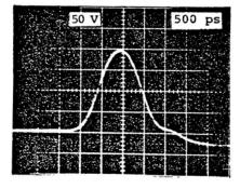
Fig, 3: Oscilloscope photographs of partial discharge currents using UWB detection. Only the electronic portion of the current is visible. (a) PD frcn either a sharp point in gas (corona pulse) or a tree in epoxy.
