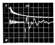
(top trace). The bottom trace shows the voltage induced on the copper conductor in a coil. A 1000:1 high voltage probe was used to measure the upper trace voltage.
