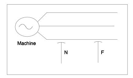
Figure 2 Schematic of capacitive bus couplers on a motor feed.
