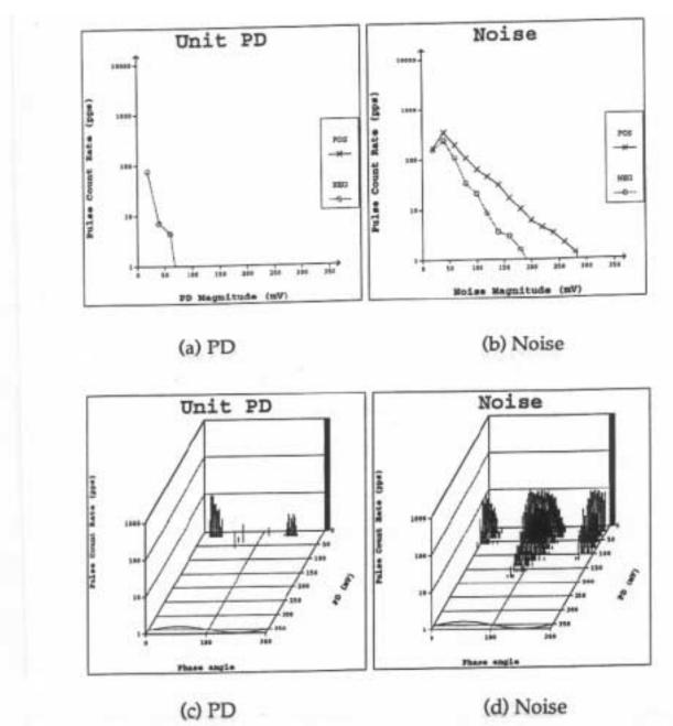
Figure 3 Pulse height and pulse phase analysis plots of A phase of an operating 6 MW stator.
