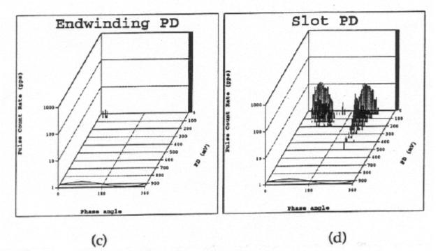
Figure 9 PD activity with the Riviera unit operating at 365 MW.
