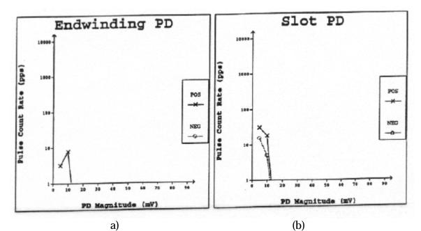
Figure 7 PD pulse height analysis plots for an SSC installed in a new 122 MVA generator.
