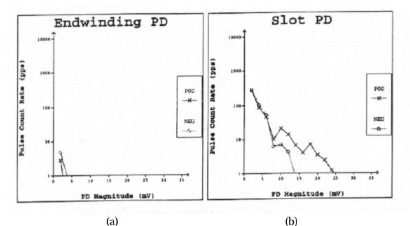
Figure 8 PD activity in the slot and endwinding with the Turkey Point Unit 1 generator operating at 460 MW.
