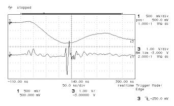
Figure 2 - PD (lower trace) recorded during a single surge (upper trace) from a surge tester.
