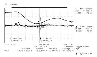
Figure 3 - 'Infinite persistence' recording of multiple PD pulses (trace 1) occurring at the peak of the surge voltage on the same motor as in Figure 4. Since the PD pulses appear as a light trace compared to the bold surge (and the surge transient recorded on the PD signal output) it is clear that most surges do not produce a PD pulse.
