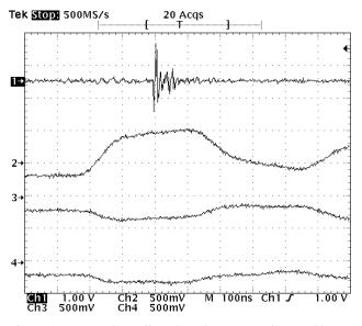
Figure 1 – PD pulse collected at the motor using a 600V IFD operating at 60 Hz. Channel 1 is PD from Phase A. Channel 2 is a A Phase Transient (divided by 2000). Channel 3 is B Phase Transient (divided by 2000). Channel 4 is C Phase Transient (divided by 2000).
