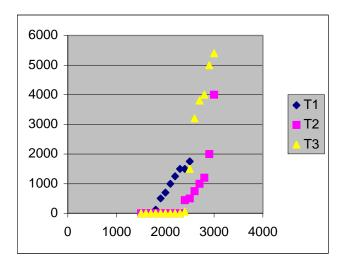
Figure 4 - PD magnitude as a function of applied surge voltage (100 ns risetime). The vertical scale is the PD magnitude from the new detector, in mV. The surge voltage (V) is the horizontal scale.
