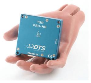
The ultra-small TSR PRO and TSR PRO-HB are portable shock recorders with built-in accelerometers. Easy to use, the TSR records for seconds to hours, writes data directly to flash memory and stores up to 2000 events.
