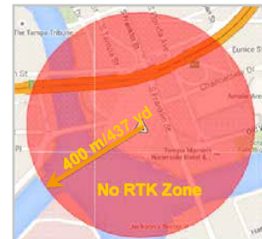
Figure 13 – 10 mW Chirp jammer without mitigation
