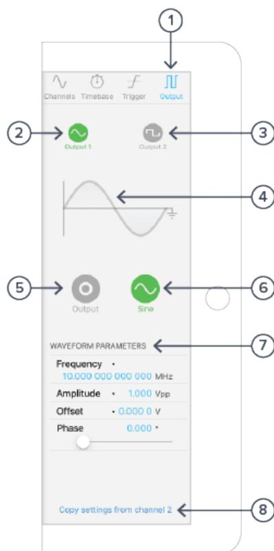
The output pane of the oscilloscope allows for generation of various waveforms on the Moku's output channels.
