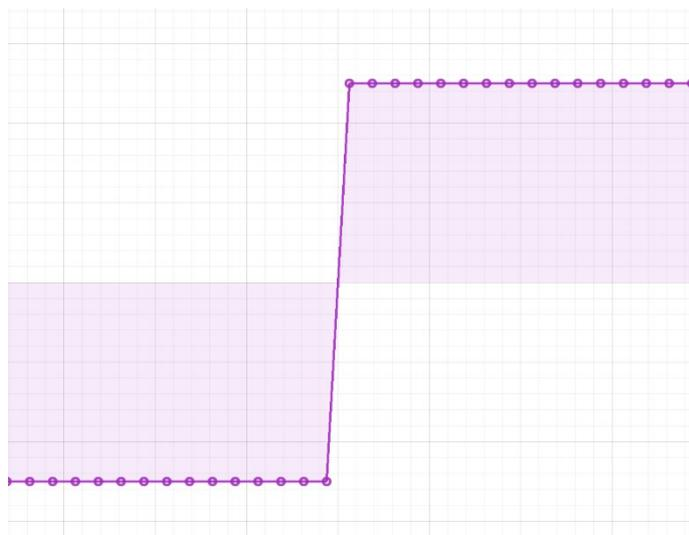
Linear interpolation does not perform any up-sampling. For display, it marks each point in the original data set and draws a straight line between them. This is “ugly” but doesn’t “invent” any new data points.
