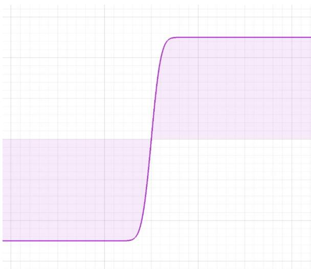
Gaussian interpolation “smooths” the signal out, preserving the visual characteristics of the signal at the expense of frequency information.
