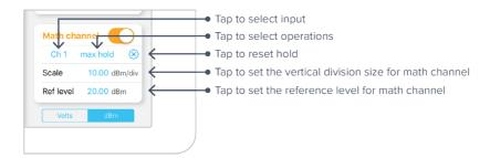
Four operations are currently supported by Moku:Lab's Spectrum Analyzer: +, ×, min hold and max hold.
