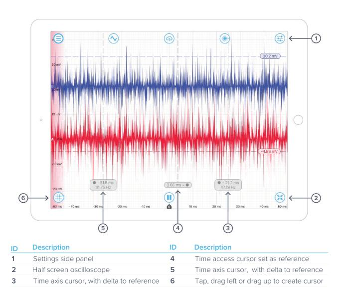
See Oscilloscope for full details of the oscilloscope user interface and controls.
