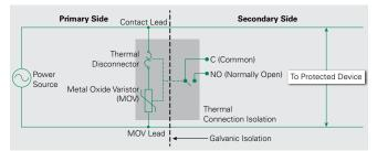
Note: This typical circuit shows how the switch pins (C and NO) can be used to indicate the connection status of thermal disconnector for remote indication. This denotes that the circuit will be no longer protected from surge currents by the MOV after the thermal disconnector forms open circuit.
