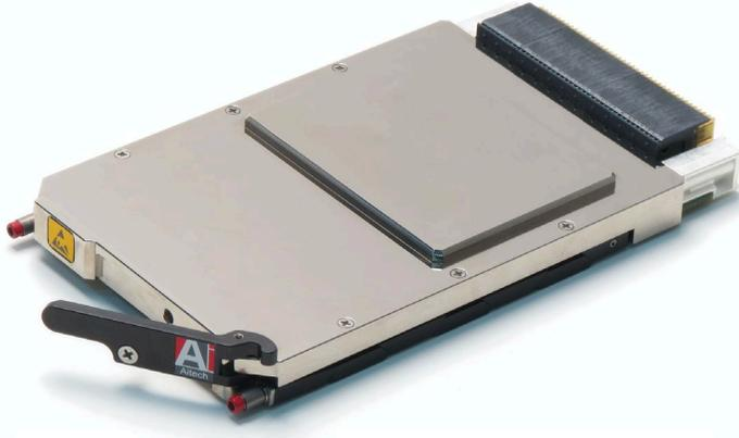
The updated C530 multi-head GPGPU is the most powerful AI (Artificial Intelligence) enabled 3U VPX GPGPU board, providing remarkable performance in a compact and rugged form factor.
