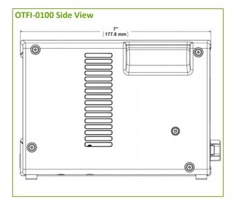
Air intake vents on rear; exhausts on sides. Do not block vents.
