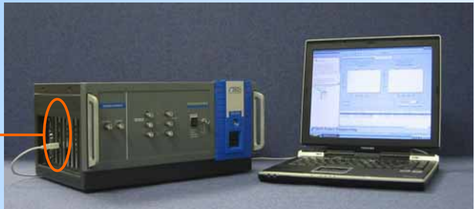
PDA-IV instrument with dual frequency option. The laptop controls measurement process and stores test results
