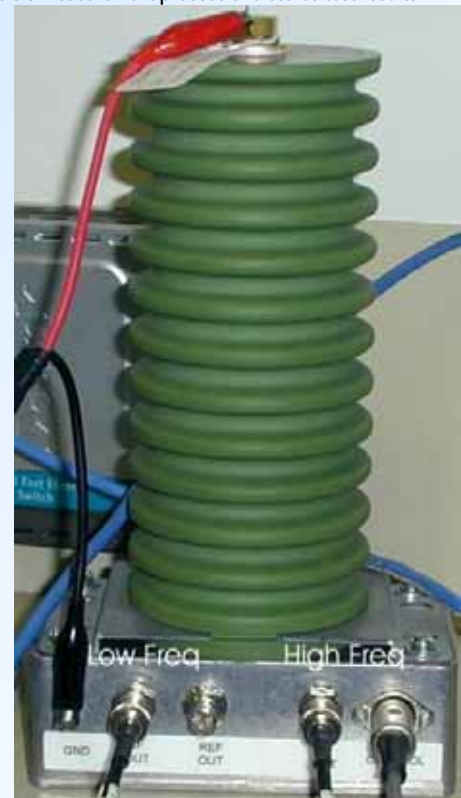
25 kV PD free coupler with low frequency option
