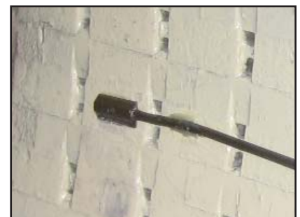
Iris Power TFProbe glued to a turbine generator stator tooth
