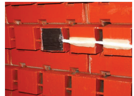
Iris Power TFProbe glued to a turbine generator stator tooth
