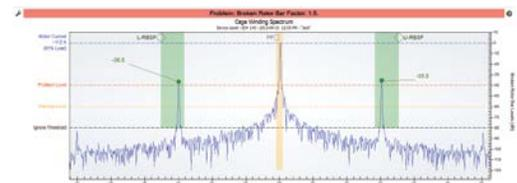
Broken rotor bar spectrum analysis
